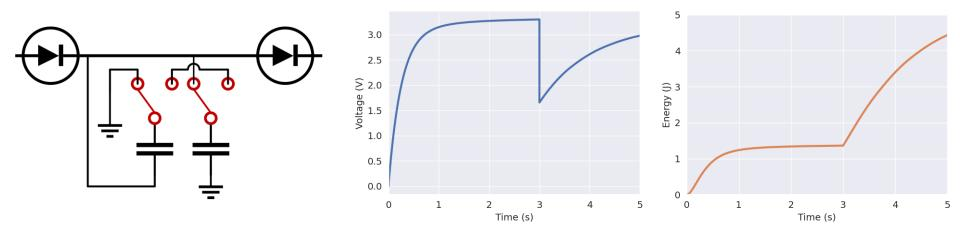
Variable capacitance/voltage without energy loss
