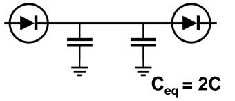
Reduce capacitance during discharge
