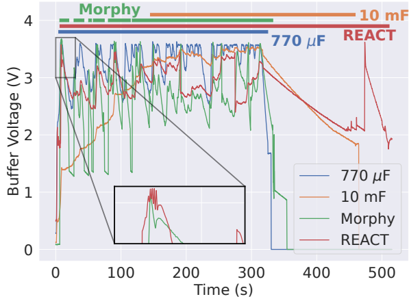
Figure 6. Buffer voltage and on-time for the SC benchmark under RF Mobile power. Solid bars indicate when the system is operating.
