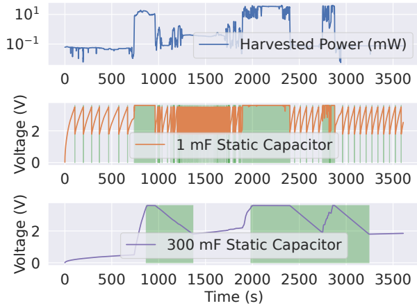
Figure 1. Static buffer operation on a simulated solar harvester. Highlighted blocks indicate the system is running.
